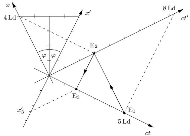
(c)  $f' = \sqrt{\frac{1 - \beta}{1 + \beta}} \cdot \frac{c}{\lambda} = \sqrt{\frac{0,2}{1,8}} \cdot 120 \text{ MHz} = 40 \text{ MHz}$
