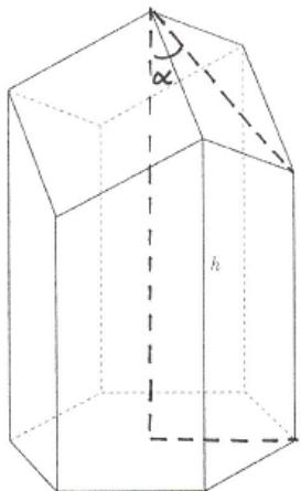
The figure shows the model of a honeycomb cell. You can see that the top is no plane hexagon. The biologist D'Arcy discovered that the surface area is just dependent of the inclination angle of the three areas forming the top of the cell. He even found a formula for this:
